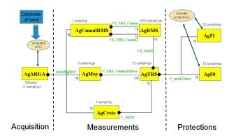
Figure 7. OASISepam: software architecture of the Sepam 10 using OASIS.
