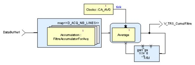
Figure 10. AgentAverage node of the SCADE model of the Sepam application.
