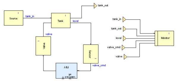
Figure 5. SCADE model for level control in a water tank.
