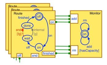
Figure 2. JavaBIP models of three routes and a monitor.
