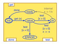
Figure 10. Example of a non-deterministic component with data
