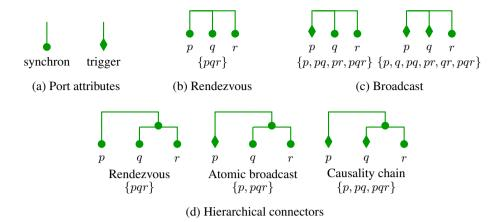
Figure 9. BIP connectors: below each connector, we show the set of interactions it defines
