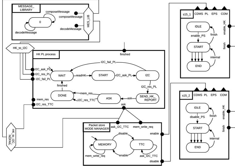
Fig. 15: Composition of Client-Server and Mode management architectures
