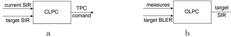
Figure 4.5: Closed Loop (a) and Outer Loop (b) components of the Power Control system.
